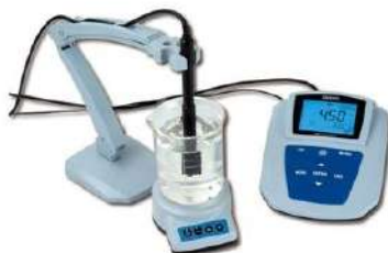
Figure 5.49 Setup with magnetic mixer and mixed needle for agitation
