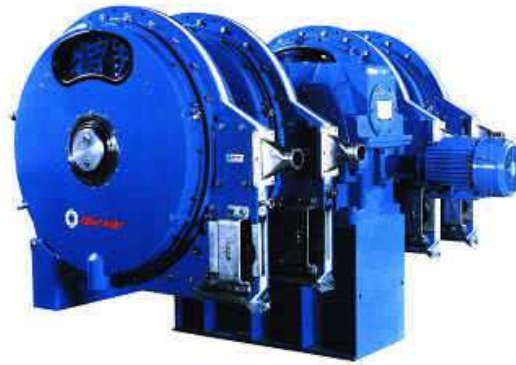
Figure 6.15 Rotary press dewatering machine (1,200φ, 4 channels)
